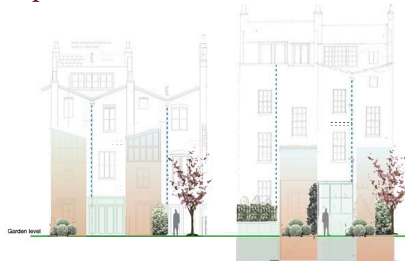
Diagram 4 - left, houses that start at ground level, right, houses that start at lower ground level.
