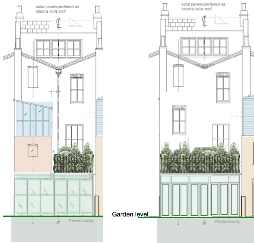
Continuous projections with uniform fenestration at lower ground or ground floors can be supported, provided minimum garden spaces remain.
